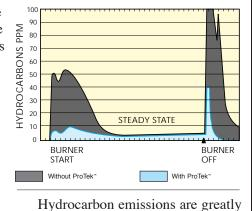
reduced when the Delavan ProTek™ Nozzle System is used. Hydrocarbons are typically elevated at start-up and shut-down of the nozzle firing, as both of these graphs show. When the ProTek Nozzle System is installed, the dramatic benefits are seen in these charts which show comparative results with and without the ProTek™ valve. Results will vary by application.
