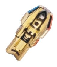
expense. You may be aware that the mesh or sintered filter section at the back end of a fuel nozzle is screwed in place. Delavan has developed a tiny "valve component" that screws into the nozzle head in place of the standard filter. The valve component is recessed within the same type of sintered filter material, so the assembled nozzle with valve is indistinguishable from a regular nozzle.
