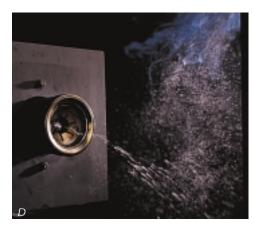
Standard nozzles drip and drizzle at shut-down, shown here in stopaction photography (C & D) timed to match ProTek photographs A & B.
